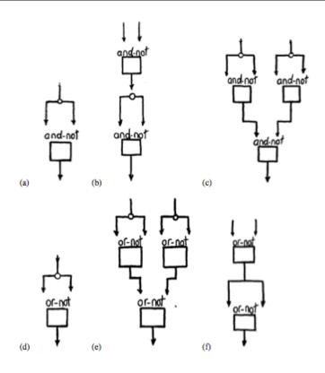
☑ 17.5 Making the three basic gates from and-not and or-not gates. (a) and (d) are not- gates, (b) and (e) are and-gates, while (c) and (f) are or-gates.(YET)
